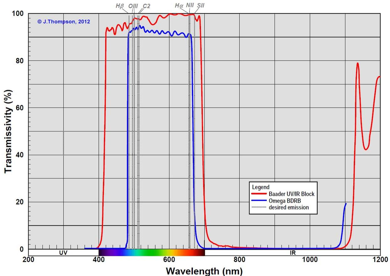
Figure 2 Spectral Response Comparison Between BDRB & Typical UV/IR Cut Filters
