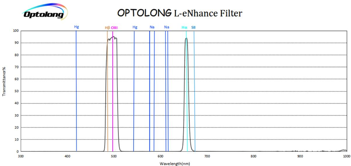
Figure 1 Spectral Response of Example Multi-Narrowband Filter
