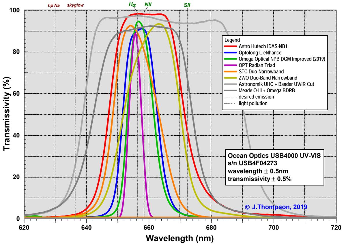
Figure 5 Measured Spectral Response Comparison – H $\alpha$  Pass Band
