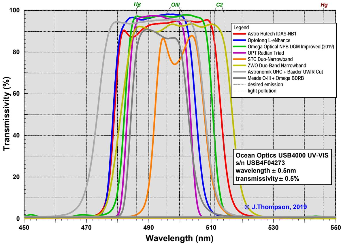
Figure 4 Measured Spectral Response Comparison – O-III Pass Band
