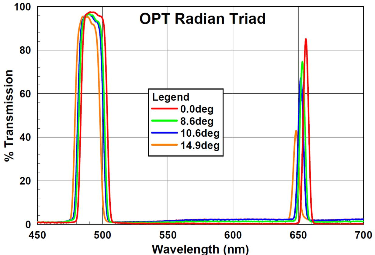
Figure 11 Impact of Filter Angle On Spectral Response – OPT Radian Triad
